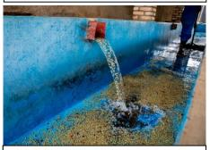
Image shows the beans passing through the flotation channels at Karambi coffee washing station
